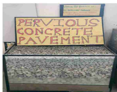
Pervious Concrete Pavement
