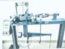
Direct Shear Test Apparatus Normal Stress vs. Shear Stress Curve
